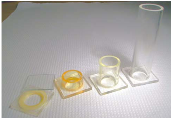
Utermohl sedimentation chambers: bottom plate with cover glass, 10 mL, 25 mL and 50 mL chambers
